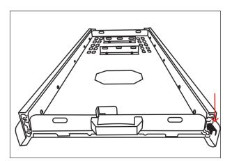
Mark the six drilling points through the slide fixing holes with a permanent marker
