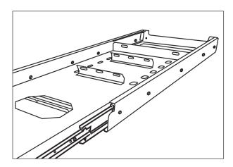
Drill six 7mm holes for the Tee Nuts
